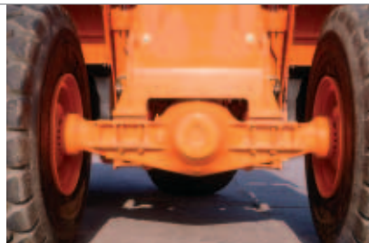
Axles generously dimensioned. Outboard planetary hub reductions to limit the torsional stresses in the driveshafts.
